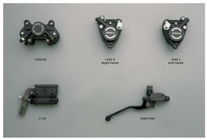
Storz Performance is a direct importer of these well-made Italian disc brake components for dirt track, road race, and drag race applications. These components are precision die cast aluminum with hard anodized alloy pistons. All calipers are dual acting and feature Ferodo brake pads that quickly detach without wheel removal. Grimeca brake calipers and master cylinders are threaded to accept 8mm x 1.0 fittings for attachment of brake lines.
